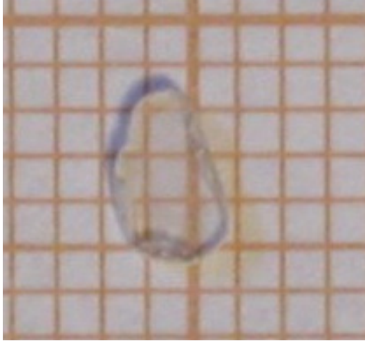
Figure 2. X-oriented \alpha -GaPO 4 plate. The smallest division of the grid is 1 mm.
